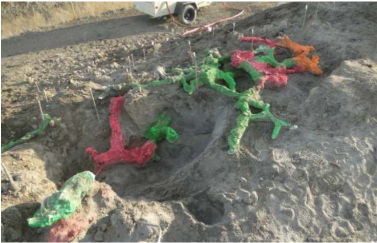
Figure 2. Photo Showing Investigation of Animal Burrowing Activity.
